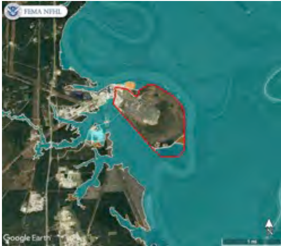
Figure 11. FEMA records showing the ash pond dam within the 100-year flood plain.
